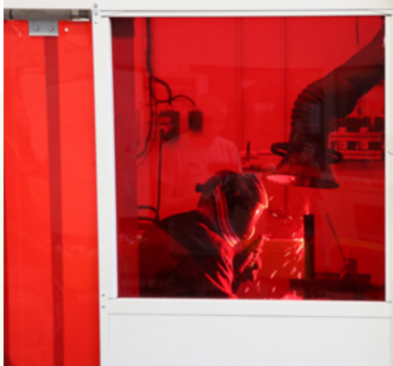
► Figure 17. A welding booth fitted with local exhaust ventilation, which extracts welding fume away from the operator. The booth is also fitted with screens to protect other persons in the vicinity from arc eye, which is an inflammation of the cornea, caused by ultraviolet radiation from the arc during welding.
