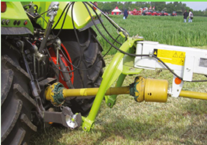
► Figure 29. Guarded power take-off shaft coupled to a tractor and the implement.
