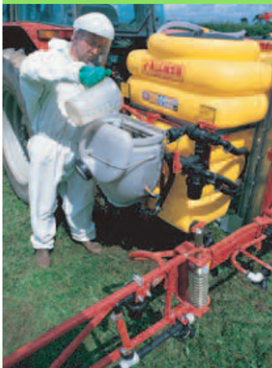
► Figure 8. A worker mixing pesticides using a low-level induction bowl placed at an appropriate height.
