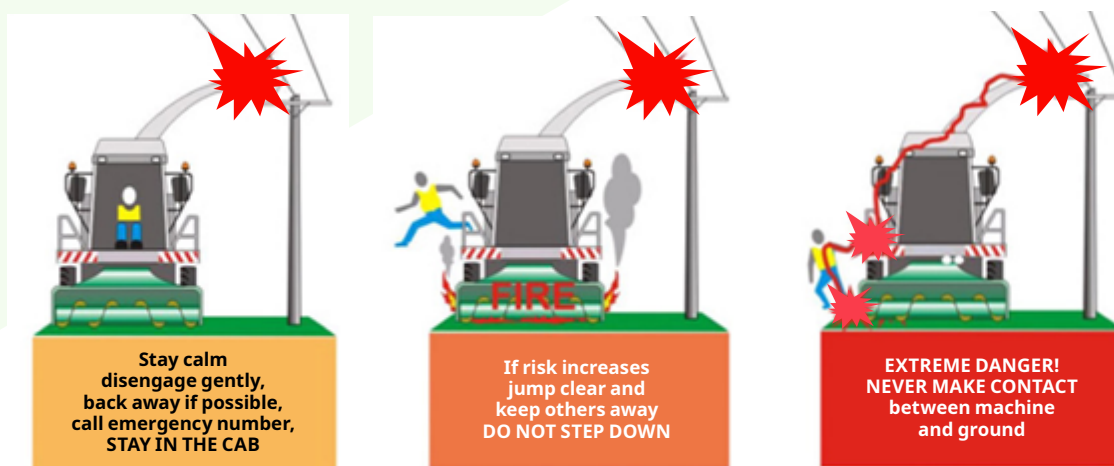
► Figure 48. Actions required if machinery comes into contact with an OHPL.
