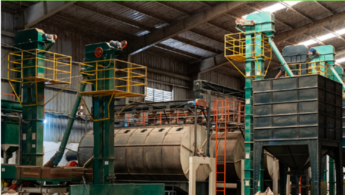
► Figure 36. Guardrails fitted to platforms to prevent workers from falling.
