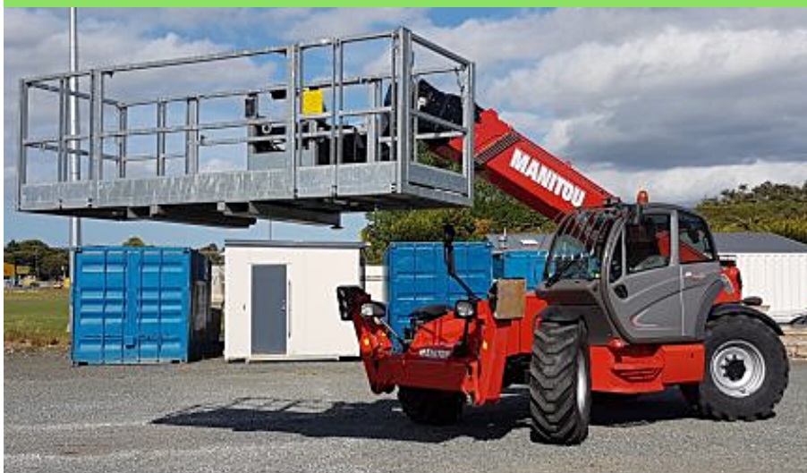
► Figure 35. Working platform on a mobile plant with 360° edge protection.
